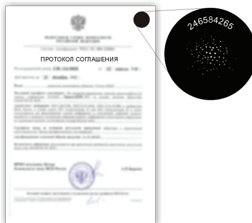
Fig. 5. Strict report document with the individual numeric code protection by electrodischarge procedure.
